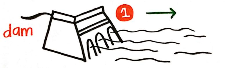
Flowing water is directed towards & used to spin giant turbines.
